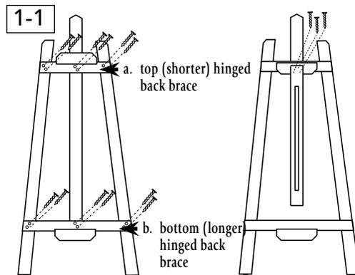
3) Attach top (See 1-1) and bottom (See 1-2) back braces to the hinged cross braces using (6) 1/4" screws through pre-drilled pilot holes.
