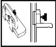
The Elevator Bolt Locking System is used on top trays on Best easels. The 2 metal plates and round plastic guide keep the parts parallel which
